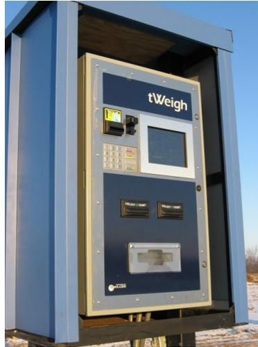
This allows a truck driver to pull away from the scale, adjust his load and check his weight again to make sure he is legal before leaving the scale site.
